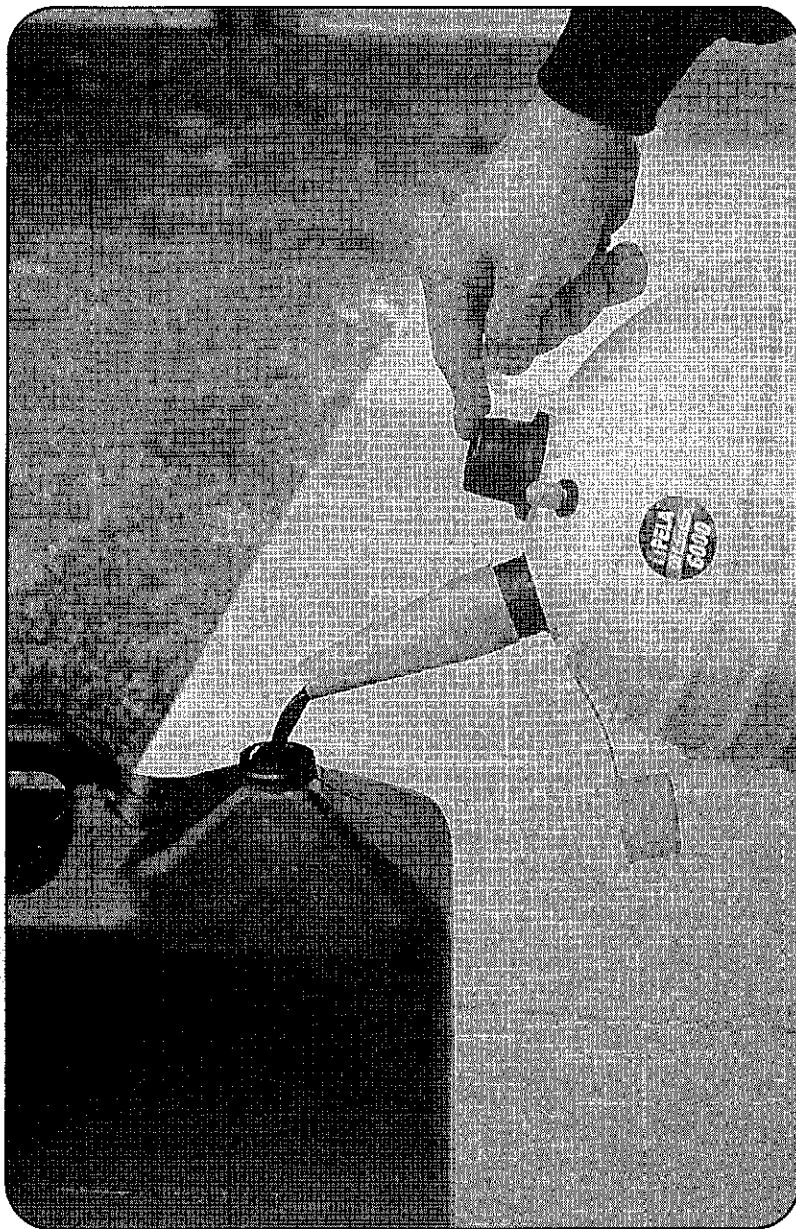
4. To drain the 1.57-gallon spherical tank, simply push on the provided funnel cone and pour the old oil into a disposal container.
